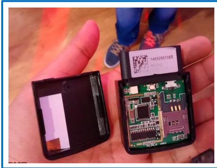
The OBD (On-board Diagnostic device) with a Jio SIM inside is attached to the OBD port of the car and thus it creates a Wi-Fi spot on the go.
